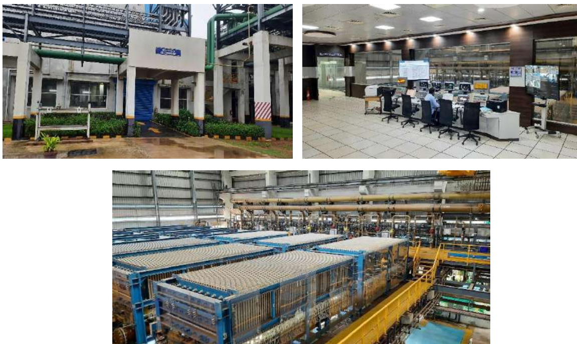
Fig 1. Membrane based Cell House Section
